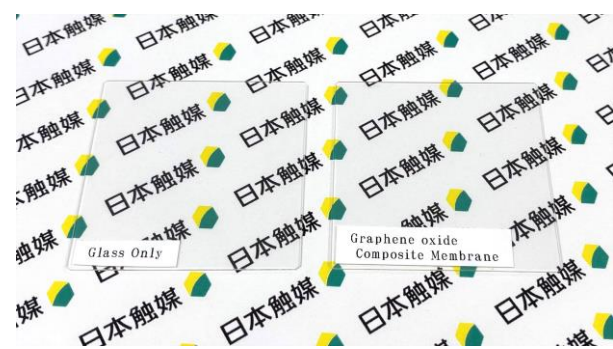
Fig. 4 Graphene oxide composite membrane on glass (transmittance of light with 600 nm wavelength: 99% or higher) Left: Pristine glass substrate. Right: After graphene oxide composite membrane treatment
