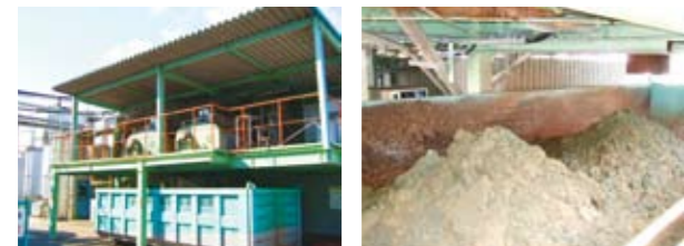
Dehydrator for reducing the water content
