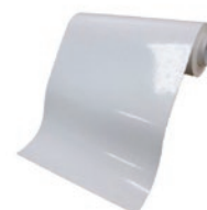
Separator for alkaline water electrolysis
