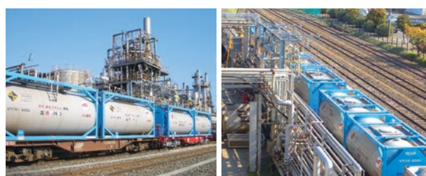
An example of modal shift (railway tank containers and loading and filling equipment)
