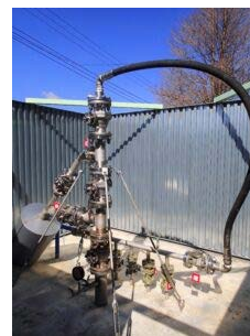
Well for extracting brine water and natural gas
